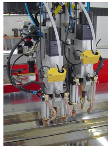
grounding by pneumatic mass clamps mounted on welding head
