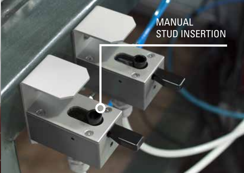
MECHANIC MASS CLAMPS MOUNTED ON WELDING HEAD
